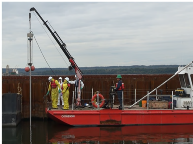
Sediment – surface and core samples collected after dredging to certify removal of contaminated sediment
