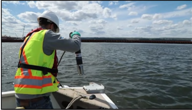
Water – measuring turbidity
